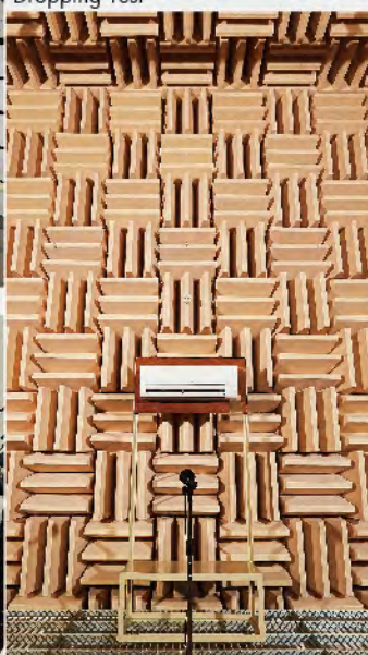
Anechoic Chamber Noise Test
