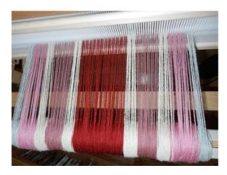
This story begins with this warp threaded through 2 heddles (12.5dpi) on my rigid heddle loom. Threading was very complex as this set-up actually produced a version of Rosepath...on a rigid heddle loom!
