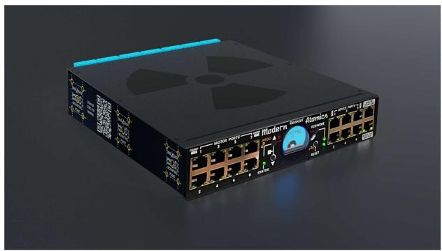
"Patented and developed by our Modern Atomics Chief Technology Officer Paul Bryson for our previous startup, NetStreams, this protocol multiplexes the networking packets along with the power delivery on just a single pair of wires. This allows basic RF pre-wired projects like the one with Desert Sun Technology to have full two-way network data and the power for the motor as if they pulled a CAT5 or multiconductor cable," says Modern Atomics Chairperson Michael Braithwaite.
