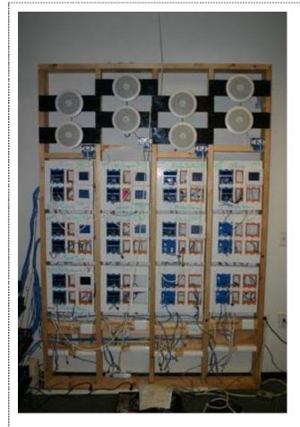
NetStreams engineered this jig to test product performance in large-scale projects. Kevin the company's CEO, said the largest known NetStreams installation is a 12-source, 70-roc system complete with lighting, HVAC, and security control. No, it's not my house.
