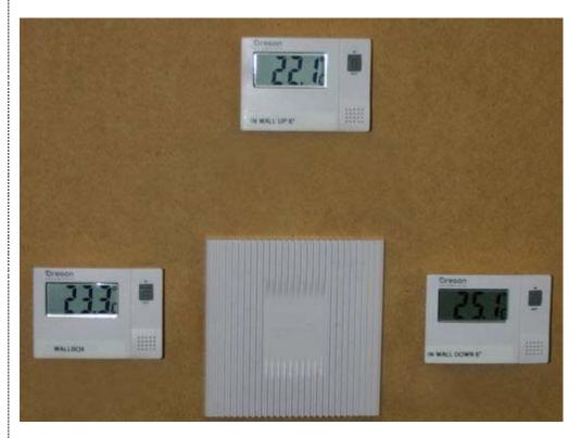
All NetStreams products endure consistent and rigorous environmental testing. This pictur the thermal testing of the company's SpeakerLinX IP-Based Amplifier/Room Controller mo inside a simulated wall. The unit plays incessantly but stays cool in an enclosure made of 1 board and stuffed with insulation. Marketing VP Petro Shimonishi says most dealers wonds amp can safely be installed in a wall. Apparently, it can.
