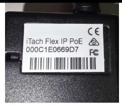
THE #FLX-IP-P will be identified in many IP Scanners as \ITACHFLEX by Global Cache
