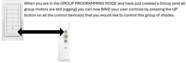
The motors will stop jogging for approximately 2-3 seconds and once the motor jogging resumes the binding is complete.
