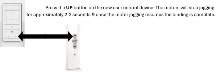
To **TEST** the binding, you can PAUSE the GROUP PROGRAMMING MODE by **TWICE** PROGRAMING MODE BY **TWICE** PROGRAMING MODE BY **TWICE** PROGRAMMING M
