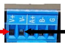
Connect the **Negative** Ground (-) from the shade motors to the right terminals marked (V-)
