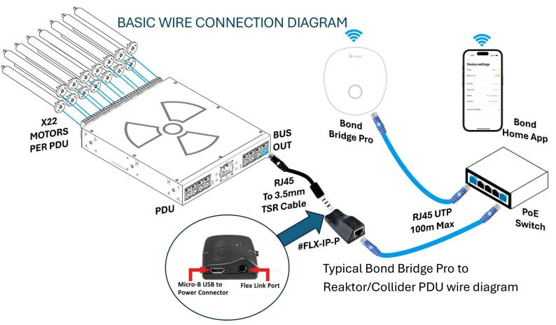
From left to right, the motors are connected to the PDU with UTP or multi conductor cabling;
