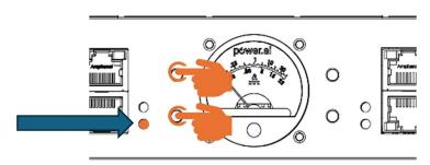
On the PDU with the #FLX-IP-P in the user mode and with the keys unlocked (You can tell the keys are unlocked when the bottom left status LED is Amber) Press and hold both the UP and DOWN KEYS for approximately 2 seconds.
