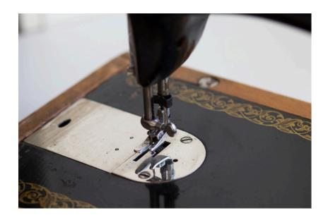
Feed dogs are located directly under the machine needle and move as the needle moves.
