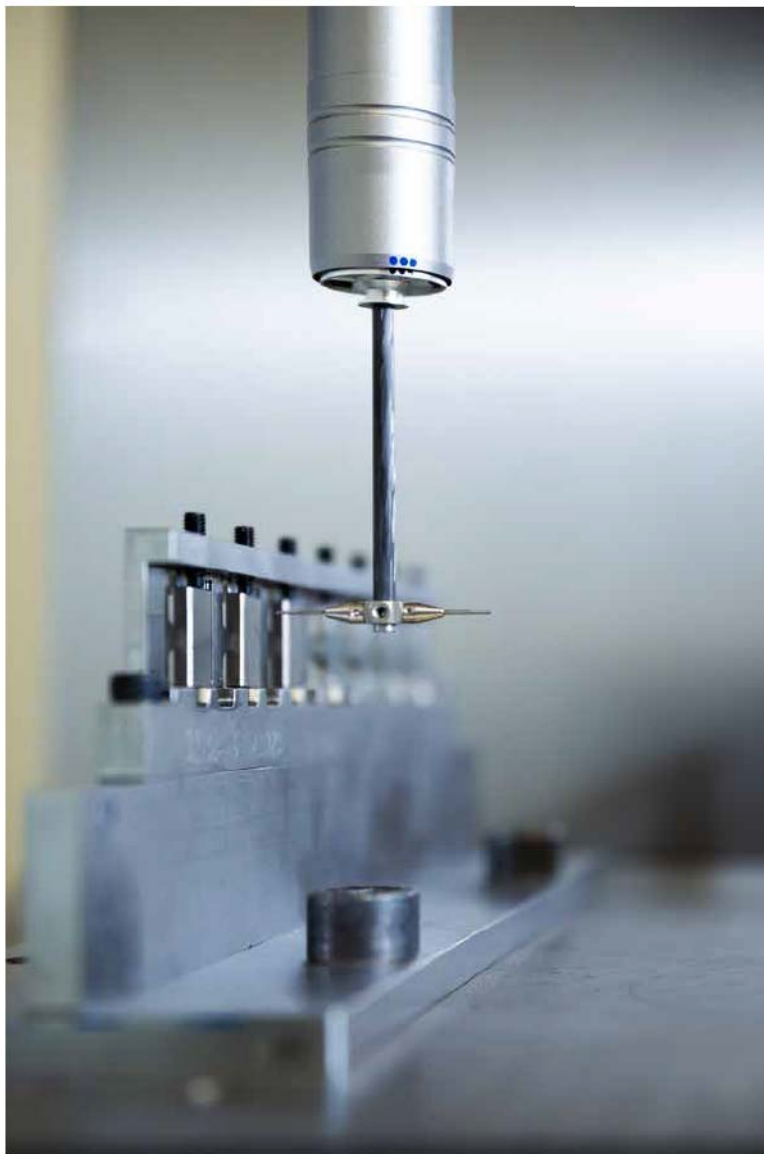
Fig. 2 Measurement and inspection of NdFeB magnets produced at GKN Powder Metallurgy's Radevormwald site (Courtesy GKN Powder Metallurgy)
