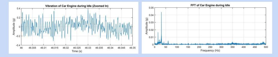
Left image: A tiny portion of a time series (idling car engine, with white noise).
