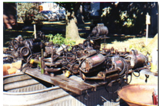
Motors to stir burgoo – Motors recycled from an earlier use in a workshop or washing machine, these motors now drive the paddles in burgoo kettles.
