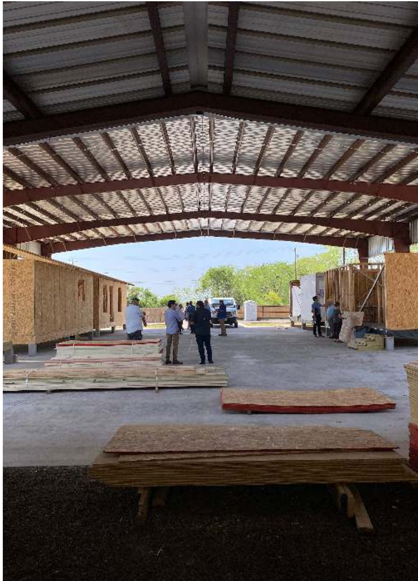
The factory requires both work stations for the boxes, and space to lay out and assemble large amounts of material.
