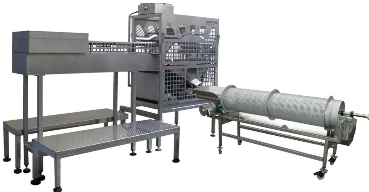
ROE RUBBER SYSTEM SHOWN WITH #723 ROE RUBBER AND #724 ROE WASHER
