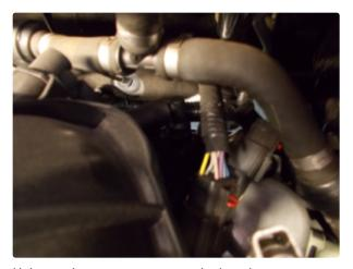
Note the earlier intake manifold versions will be aluminum and the later plastic, but we still will be installing between the intake manifold vacuum barb connecting to the outer valve on the RX can, and the valve cover PCV barb to the center of the can. This will look similar to this when removed: You will need to be careful with the line (similar to but not exact as below left) to make sure you can connect the included barbs to it and the can lines.
