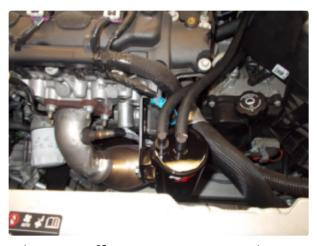
Note: There may only be room for one bolt. This is sufficient to secure the can. Above right shows the finished installation. Draining the can should be done every oil change or 5,000 miles and the oil disposed of properly as with any drain oil.
