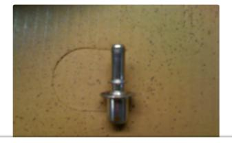
As you can see above, the original OEM hole size causes crankcase pressure to buildup and oil ingestion through the "clean side" of the PCV system upstream of the throttle body.
