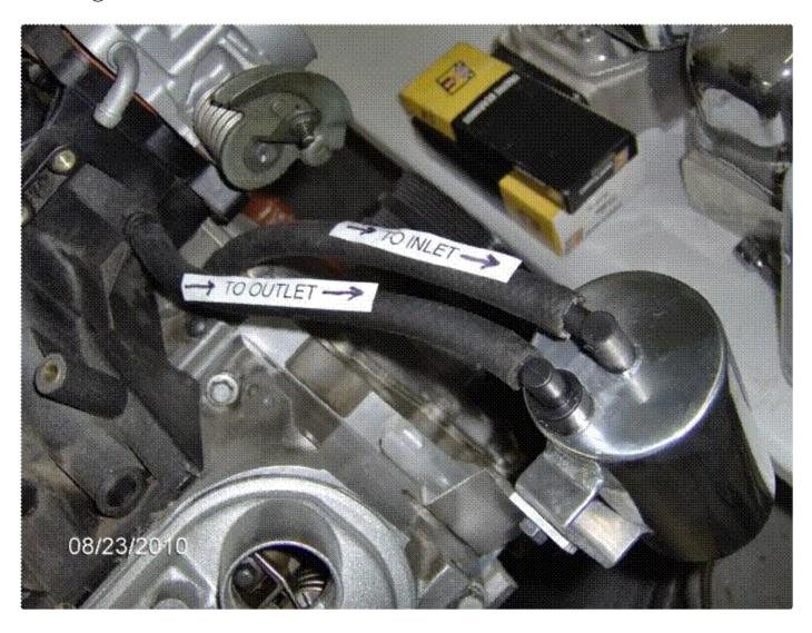
Below is an example of a dual can setup for race applications where the
