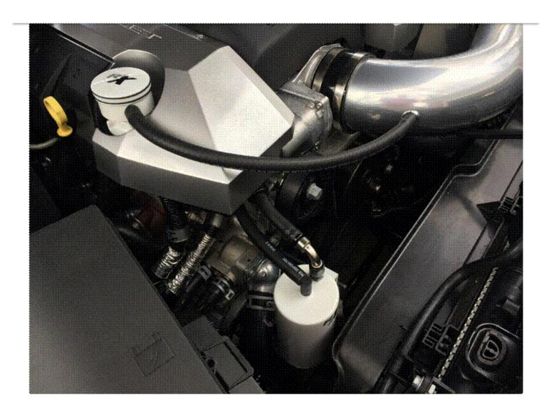
Note: Dirty side (foul vapors from crankcase) may be from valley cover OR rear of drivers side valve cover. You can "T" both together and then run to center (inlet) of RX separator can.
