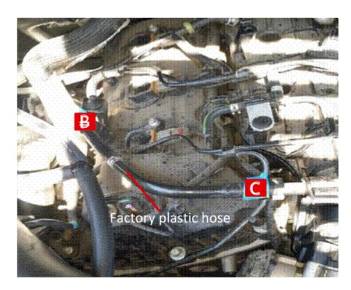
Locate the passenger side valve cover and remove the factory plastic hose
