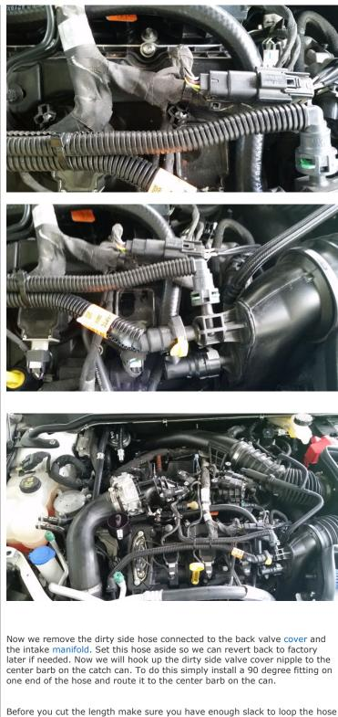
Before you cut the length make sure you have enough slack to loop the hose without crimping it. I decided to run this hose toward the passenger side of the car looping to the center barb on the catch can. Lube the center barb with WD40 and push the hose in place.
