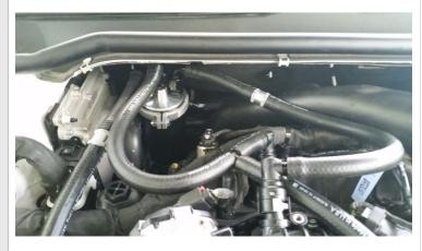
I guess I should mention I test fit the engine cover between each hose install to ensure I didn't have an obstruction or any sort. Man I love this drive by wire system no linkages or moving parts to get in the way.
