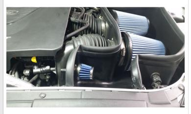
Ok before anybody starts yelling about blocking air flow I confirmed the filter is above the inlet for the fresh air and is NOT blocking air flow. Now all I have to do is slide the hose on the nipple and route it to the clean air filter oil fill breather on the motor.
