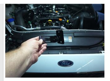
Hmmmm, something is off. Well crap the catch can bracket was ¼" to high and the bracket needed to be moved about 5/8" toward the computer to allow the can to mount. Hick up three just showed up. Moving the mounting bracket away from the mounting bolt on the 16ga plate resulted in no support due to the lack of rigidity in the mounting plate. Mounting plate version 2.0 corrects this issue and will allow for a solid support system.
