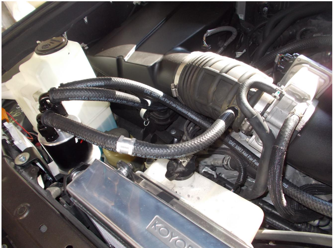
Above you can see there are some weld dimples in the core support, drill a 3/8" hole and use the included bolts and washers to secure the medium L bracket. Also, make SURE when sliding the clamp up over the can you spread the gap with a flat blade screw driver to avoid scratching the finish.
