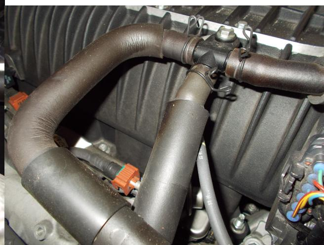
This will be replaced with a single length of hose that bridges both together with no T in it. Then you will replace the oil fill cap with the CSS (cleanside separator) and run a hose from it to the barb located on the backside of the main intake air tube that used to T into the OEM bridge hose you just removed.
