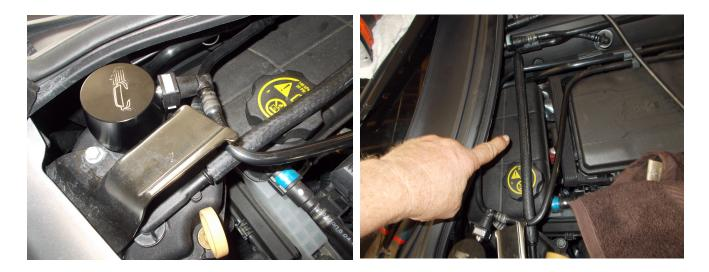
Now re-install the hood air deflector and make sure all connections are secure and the drain valve is closed on the can. Check the can to determine the amount your engine is trapping and you can most likely go from 2,000-5,000 miles (depending on how driven) before it needs to be emptied. Please dispose of the contents as you would any drain oil in proper recycling tanks at most auto parts stores.
