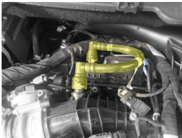
Figure 2: Step 1 of Preparation. Line connecting PCV and Intake Manifold to be removed.
