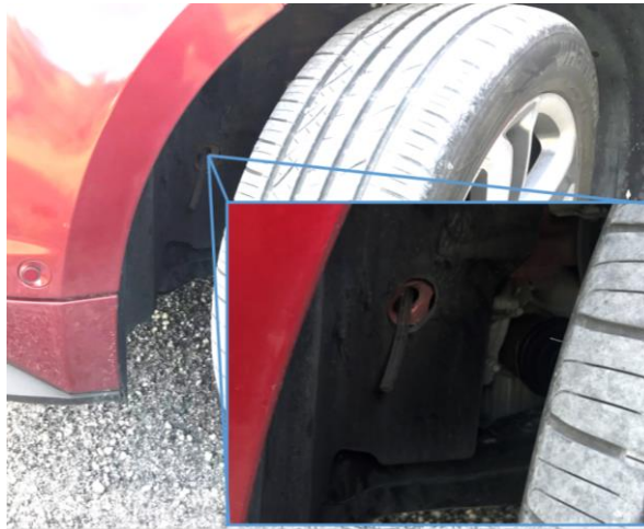
Figure 9: Drain Hose Location
