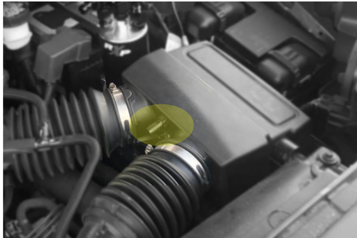
Figure 5: Completed Clean Side Separator vacuum port at airbox
