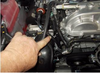
One outer fitting on can w/checkvalve flowing away from can will connect to the hard line coing from the turbo inlet.
