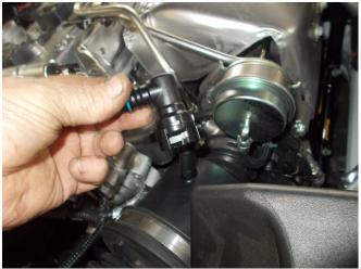
In the above left picture, you will remove the entire stainless braid and plastic tube assembly. Grasp and pull firmly and they will separate. The 90\* fittings we supply will snap onto the factory barbs. These should come precut and plug and play the correct length.
