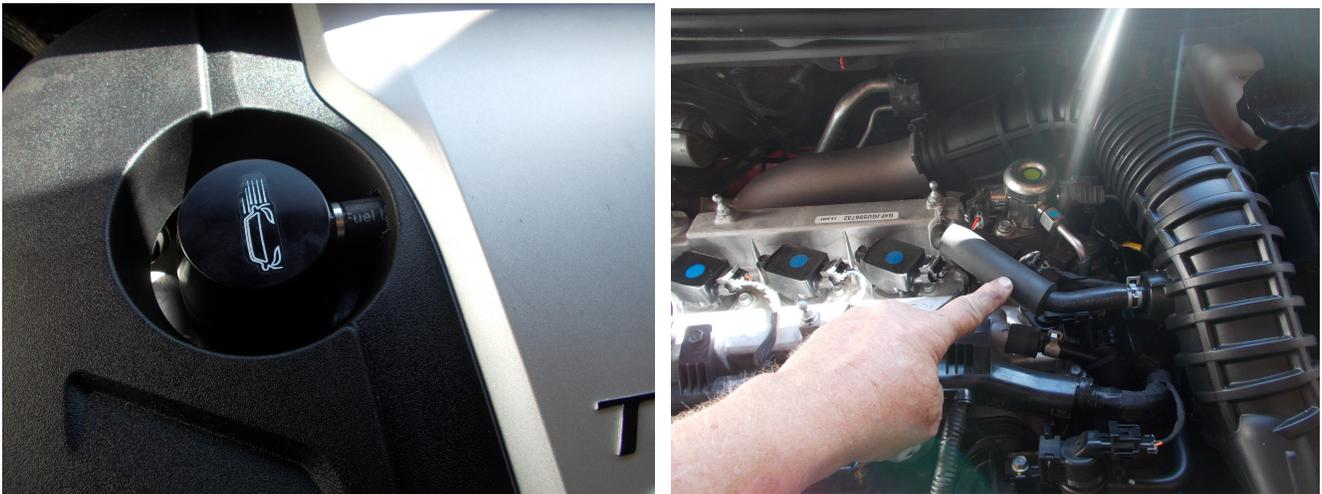
Locate the 2 main hoses we will tie into. First is the cleanside line, and this will need to be removed. Save this if you desire to revert back to stock in the future. You will replace you oil fill cap with the new base and billet cleanside unit. The billet unit will simply push into the base and seal with the 2 O rings so to add oil in the future, there is no need to unscrew the base. Make sure to grasp the base so it will seat tightly when installing.
