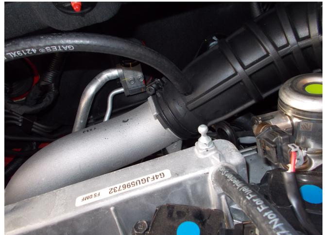
You will run the front fitting hose from can w/checkvalve flowing away from can to the hose you pulled free from the PCV valve. This provides the vacuum from the intake manifold for non-boost evacuation.
