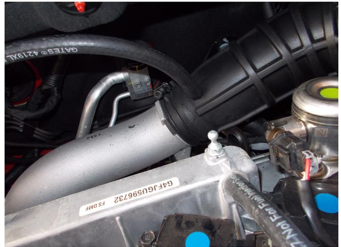
You will run the front fitting hose from can w/checkvalve flowing away from can to the hose you pulled free from the PCV valve. This provides the vacuum from the intake manifold for non-boost evacuation.
