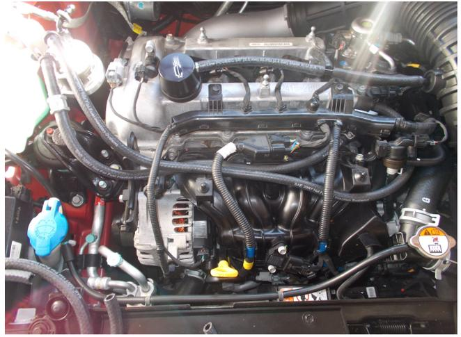
Next you will disconnect the foul/dirty side line from the factory PCV valve. The valve will be retained as this regulates the rate of flow. A hose will run from the center fitting of the can directly to the PCV valve barb. NO checkvalve on this line. (above right)
