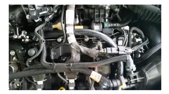
There are a couple ways to remount this MAP sensor in the catch can layout. Tracy's video shows him rerouting it on the dirty side of the engine (there was NO clean air breather installed on that video) and I was going to mount it back in the clean side run like it was initially but decided to follow Tracy's instructions to the letter. Why reengineer something that is proven to work.
