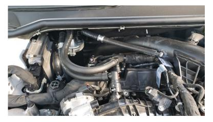
You will have to Tap the cold air tube. Tracy provides everything you need to do install. When tapping just remember not to run the tap all the way in as it will create a threaded hole bigger than you threaded elbow!!! Simply thread it enough to get threads in your tubing.
