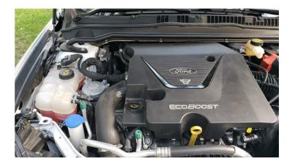
Routing the drain tube is up to you originally I routed it down behind the steering linkage and out the belly cover but when reinstalling this time I ran it down and out along the inner wheel liner and zip strapped it to the liner vai a single hole I drilled to allow the zip tie through. Easy to reach for draining now.
