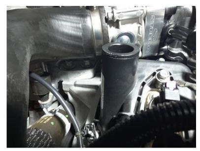
Now we are going to route the clean air hose from the barbed adaptor we installed in the CAI to the breather cap barb. Lube both barbs with WD-40, install hose on the CAI barb the route the hose along the front of the car to the clean side breather. Make sure you leave enough slack in hose to allow a clean bend to the breather. This will give you enough slack to remove the breather and set it on the front air inlet cover when adding oil.
