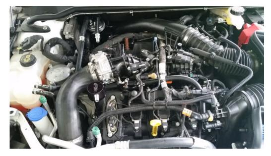
Now we remove the dirty side hose connected to the back valve cover and the intake manifold. Set this hose aside so we can revert back to factory later if needed. Now we will hook up the dirty side valve cover nipple to the center barb on the catch can. To do this simply install a 90 degree fitting on one end of the hose and route it to the center barb on the can.
