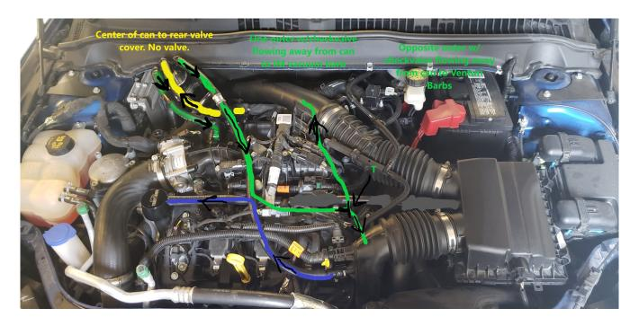
Here is the diagram that shows how the Venturi barbs need to be installed. Carefully cut the end the protrudes into the air flow as show:
