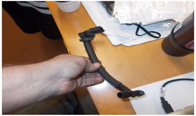
Note!!! With the 2016 and newer you may need to T this into the cleanside hose to prevent the check engine light. Sensor MUST be zip tied above the hose it is T'd into so no oil drops can get to the sensor.
