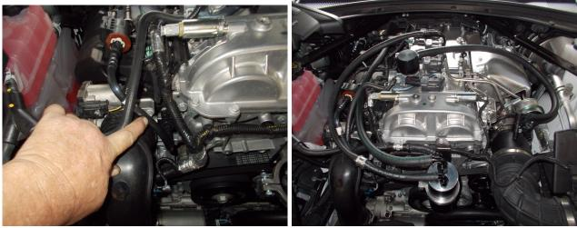
Finally make sure the drain valve is closed, and start and make sure there are no vacuum leaks. Reinstall the plastic cover and install the CSS oil cap base, then push in the CSS itself:
