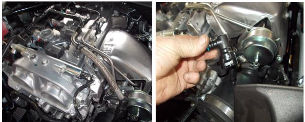
In the above left picture, you will remove the entire stainless braid and plastic tube assembly. Grasp and pull firmly and they will separate. The 90\* fittings we supply will snap onto the factory barbs. These should come precut and plug and play the correct length.
