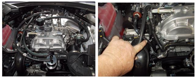
One outer fitting on can w/checkvalve flowing away from can will connect to the hard line coming from the turbo inlet.
