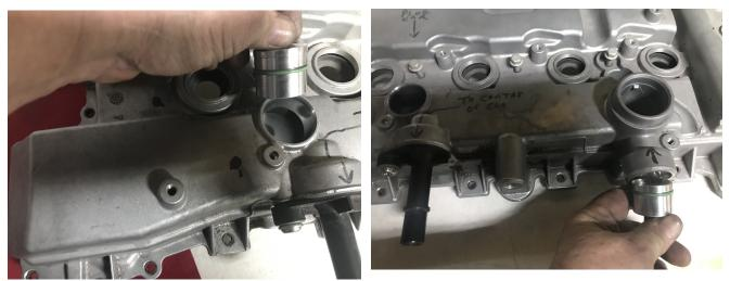
In the above left picture, you will remove the entire stainless braid and plastic tube assembly. Grasp and pull firmly and they will separate. The billet plug we supply will push into place and seal this as we are using a different routing for a more complete flushing and evacuation of the entire crankcase.
