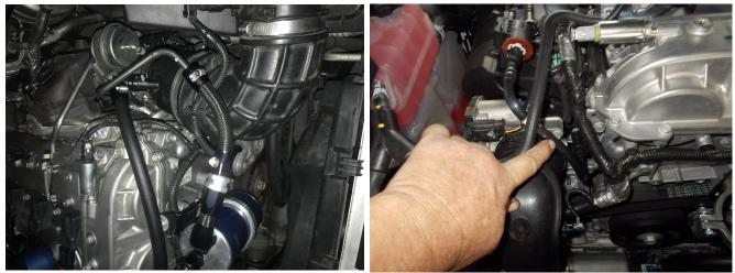
One outer fitting on can w/checkvalve flowing away from can will connect to the hard line coming from the turbo inlet. It is silver stainless steel. This takes 3/8" hose. Note the steel line can pivot.
