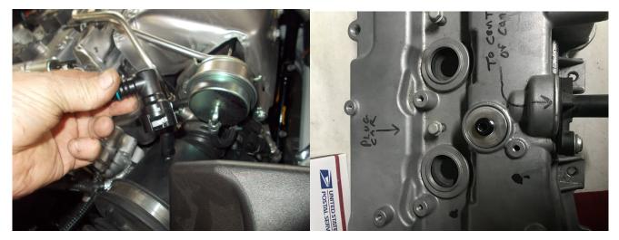
Above right shows the plug in place and the plastic fitting and barb that you will snap on one of the connectors we include and run this straight to the center of the can with no valves inline.
