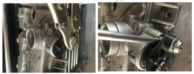
The rear most barb on the passenger side will run straight to the center of the can. No checkvalves. This you will also put a T in this hose and connect the 1/2" barb from the second billet adaptor barb. You will now run a 1/2" hose direct from the OEM barb on the air intake tube to the CSS barb (CSS replaces the stock oil fill cap). We include the OEM connector so you can save your stock tubes.
