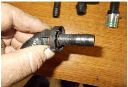
Note, the left most barb will now press into the OEM connector that did connect to the rear of the valve cover. Here is what it looks like after inserted. You may use a drop of super glue to secure it, but it will seal without.
