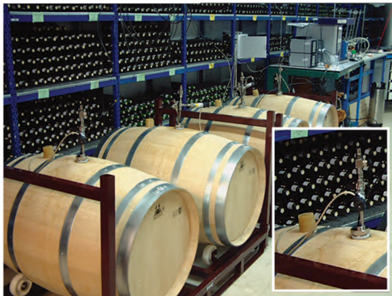
Figure 1: four American oak barrels were tested 23 times within one year to determine the evolution of oxygen uptake velocity, which demonstrated in a slowdown of the oxygen transfer rate. An airtight bung (inset photo) was created to introduce two optical submersible dissolved-oxygen probes, a gauge for vacuum measurement, inert gas inlet (N 2 ) and gas outlet to evacuate dissolved-oxygen content in a synthetic wine before every test.
