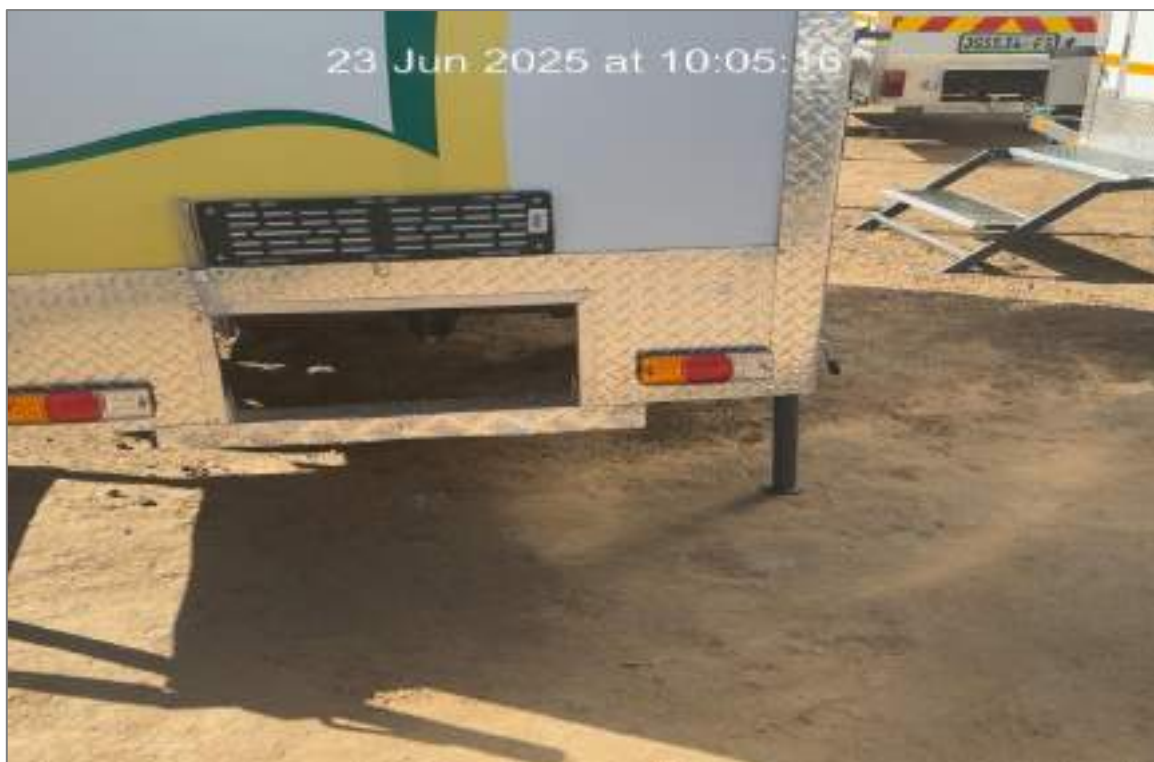
Figure 3: Chemical toilet with no drip Tray underneath.
