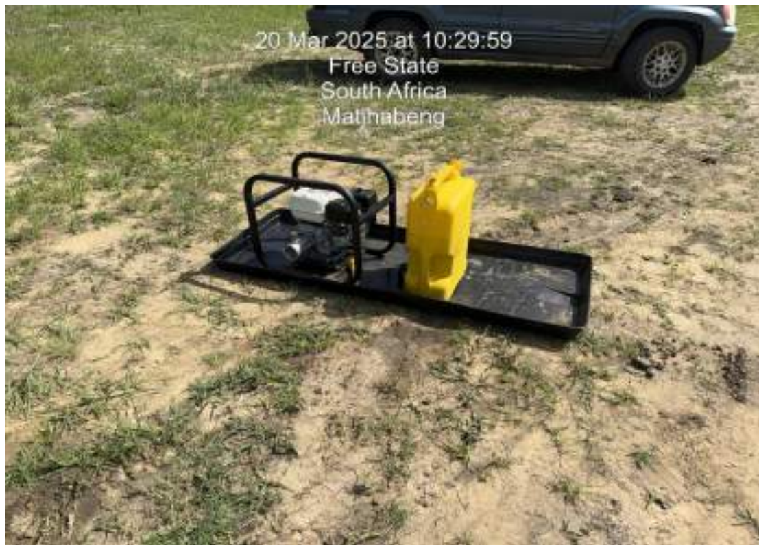
Figure 3: Drip Trays being used onsite.
