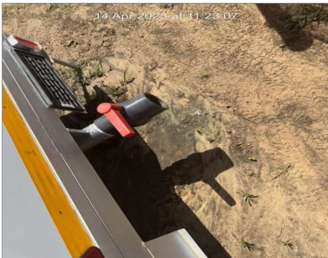
Figure 4: Spillage from the toilet
