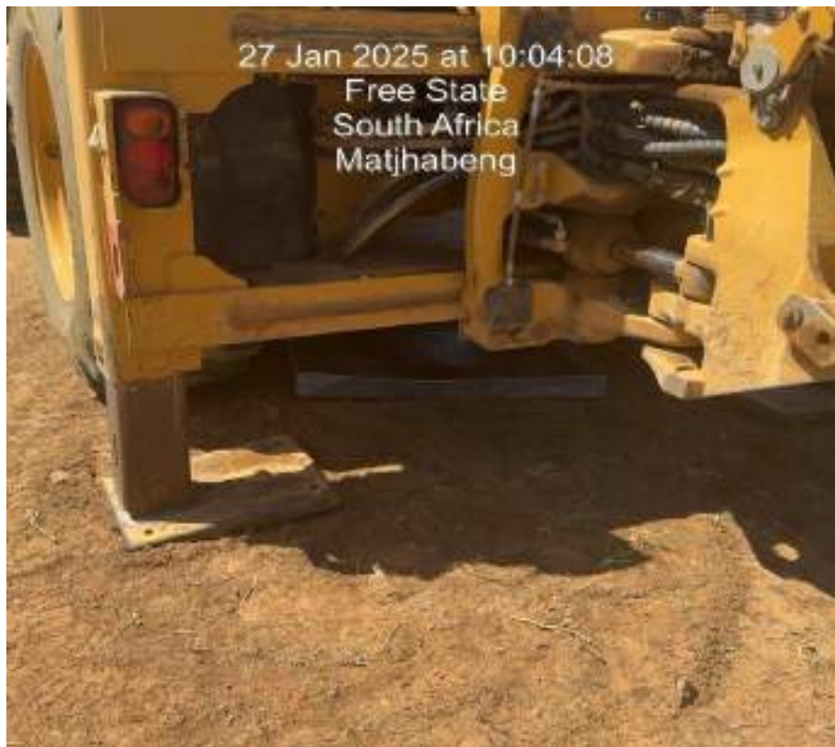
Figure 3: Standing Equipment with drip trays.
