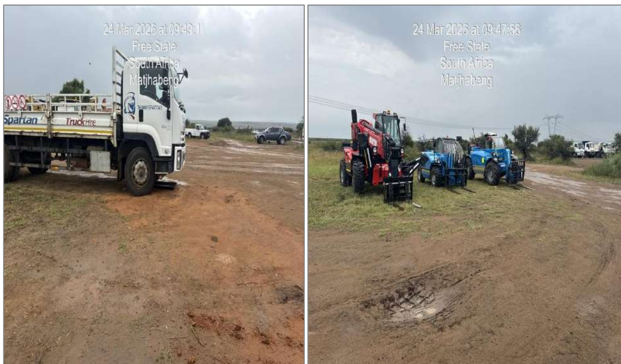
Figure 9: Equipment without Drip trays
