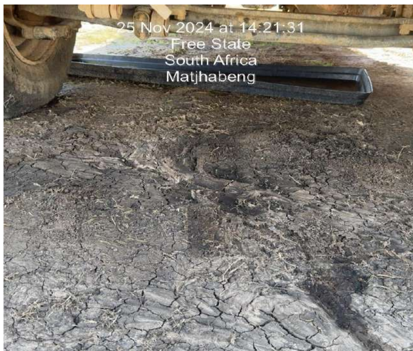
Figure 4: Equipment with drip trays
