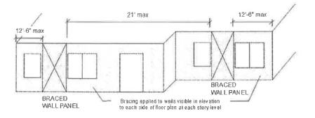
\*A braced wall panel can be anything from one-half to one brace panel.
