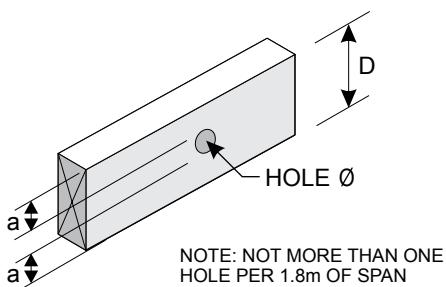
'a' min 5 Hole dia. Hole dia. max D/8
