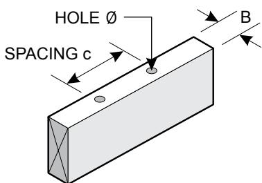
Hole dia. max 14 mm and outside middle 1/3 of beam span
