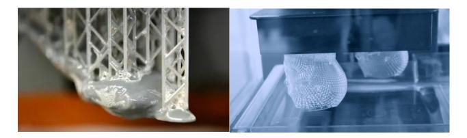
The benefits of SLA include high part precision, very fine detail, smooth surfaces and high dimensional tolerances. Some of the downsides are that SLA does tend to take longer to print than FDM, the parts are generally fragile (depending on material used) and costs are generally higher as the machines are much more complex than the relatively simple FDM printers.
