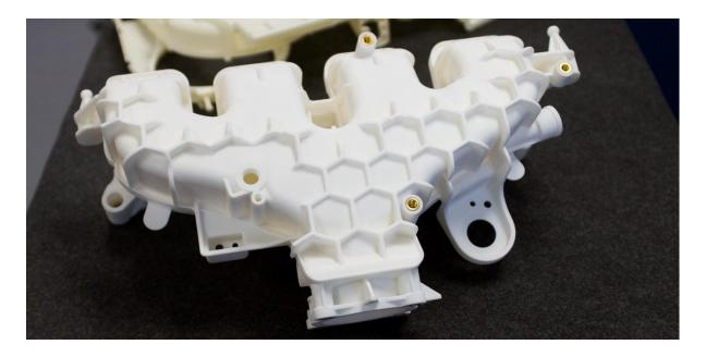
Benefits of SLS parts are that they need no support structure (so are cheaper to clean up), its fast, has good layer bonding and produces very complex and detailed parts.
