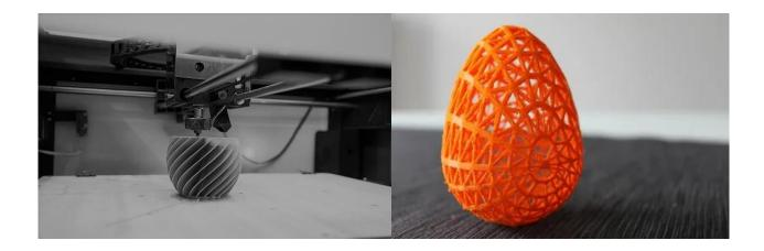
FDM parts are great for a looking at the shape and form of an objects and can also be produced to represent the durability and strength of an object, although this does depend on the material used. You can even print food (chocolate is a favourite)
