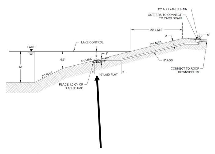
Construction fabric should be placed under the riprap at the pipe outfall into the lake. There should be 4"-6" diameter riprap 12" side around each side of the outfall.
