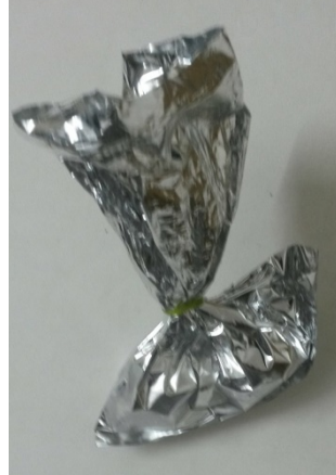
Foil pouch (coextruded, heat shrinkable, multi-layer, polyolefin)
