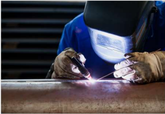
A man doing welding on stainless steel
