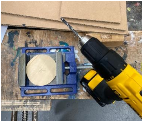
Then I marked the centre of the wheel and drilled the centre to create a hole.
