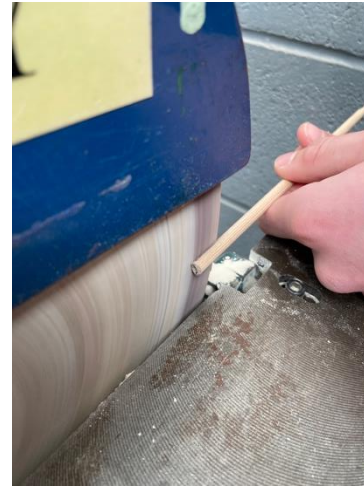
Here I am using the disc sander to sand my dowel to the correct size.
