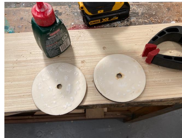
10. I used pva wood glue to stick together the 6mm wheels and I used a spring clamp to apply pressure. I left to dry overnight.
