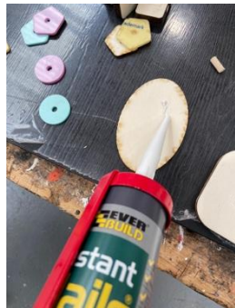
13. As I had different materials to stick together, I applied instant nails to various bits of acrylic and plywood. I put spring clamps on overnight to apply pressure.
