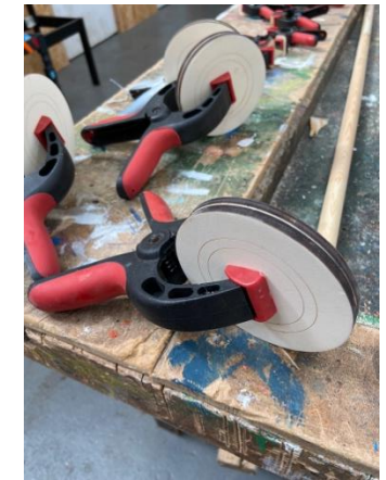
10. I used pva wood glue to stick together the 6mm wheels and I used a spring clamp to apply pressure. I left to dry overnight.
