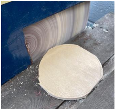
Then I sanded the wheels (health and safety: goggles, apron and extraction).
