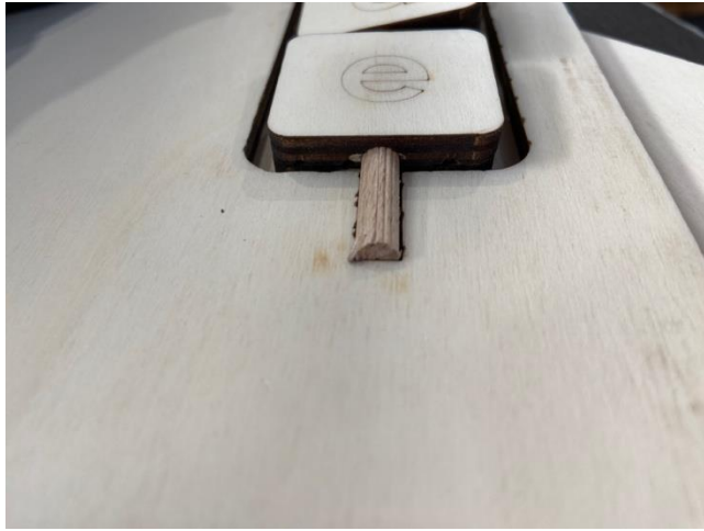
8. The dowel slots into the laser cut plywood but sticks up too far.
