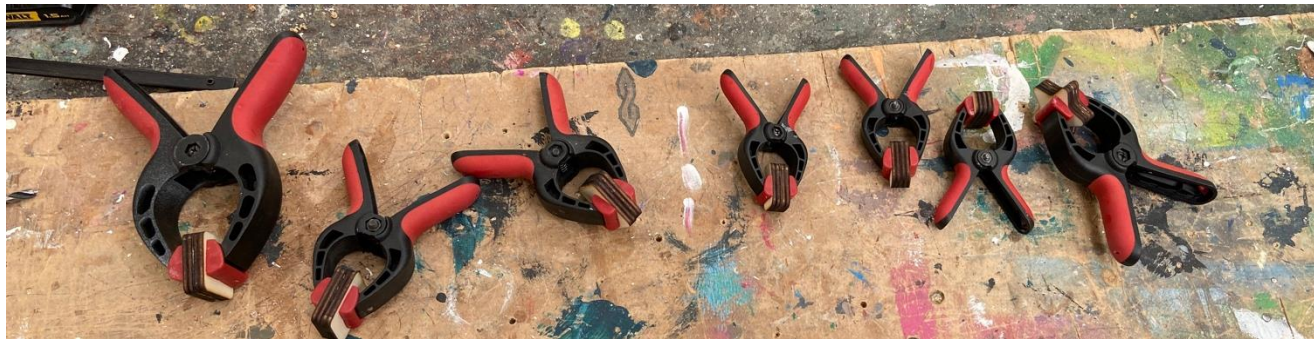
13. As I had different materials to stick together, I applied instant nails to various bits of acrylic and plywood. I put spring clamps on overnight to apply pressure.
