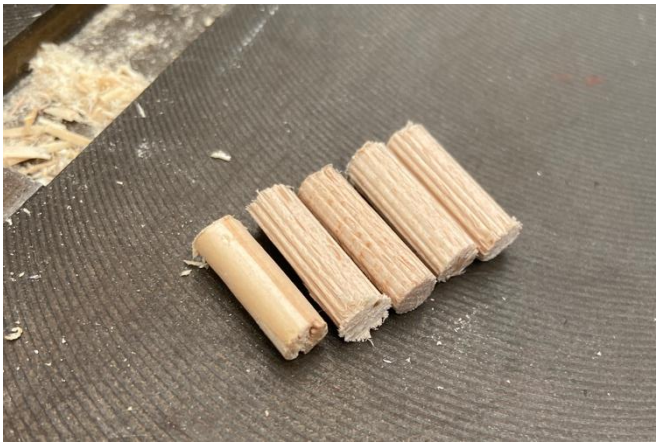
9. I marked and cut my dowel using a bench hook, a pencil and a tenon saw. These will be used as handles for my jigsaw shapes.
