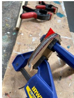
13. As I had different materials to stick together, I applied instant nails to various bits of acrylic and plywood. I put spring clamps on overnight to apply pressure.
