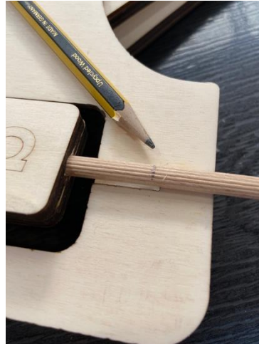
So, I marked up where to sand half of the dowel away.
