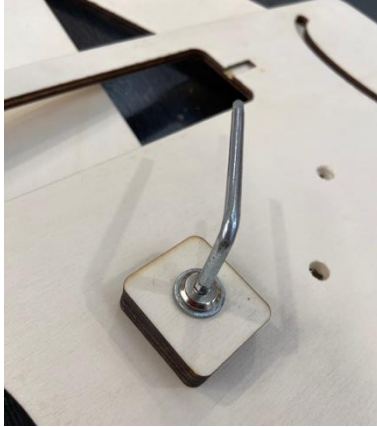
Then I used an allen key to tighten the screw for my wooden blocks. The wooden blocks fill the gap to ensure the gears and star are fixed in the correct position.
