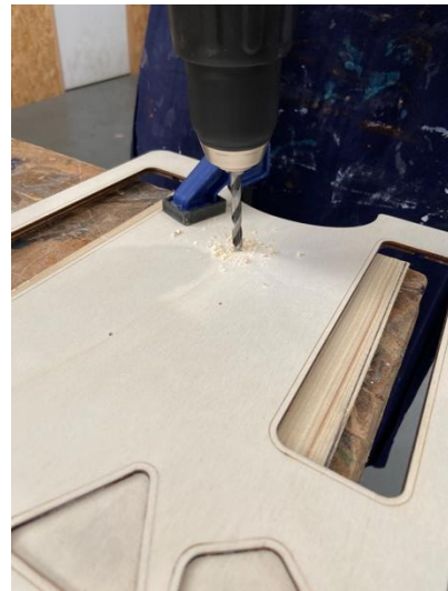
12. I drilled 8mm holes on the activity board for the gears to be fastened to.
