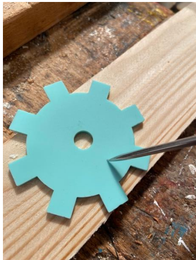
Then I use a scribe to make a small indent to where I was going to be drilling.
