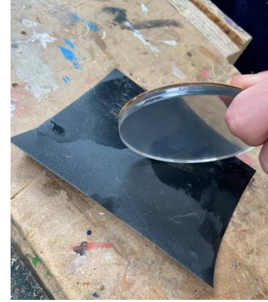
15. I used wet and dry cloth to remove the scratch marks on the acrylic mirror.
