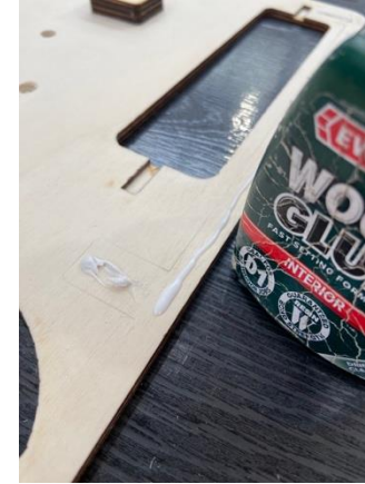
I also added a very thin line of pva wood glue around the edges.
