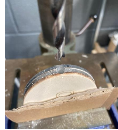
16. I tightened my blocks and mirror with a hand vice and drilled a 6mm hole with a pillar drill into each side. I used cardboard to stop the materials from scratching.
