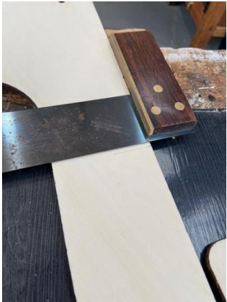
11. I used a ruler and Tri square to mark out where to put my L shaped bracket.
