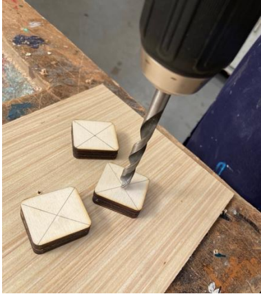
14. I marked the centre with a cross and drilled a 6mm hole in the centre.
