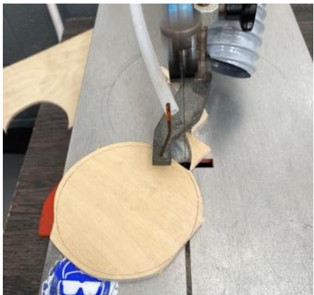
Then I used the scroll saw to cut out the wheels from plywood (health and safety: goggles, apron extraction.)
