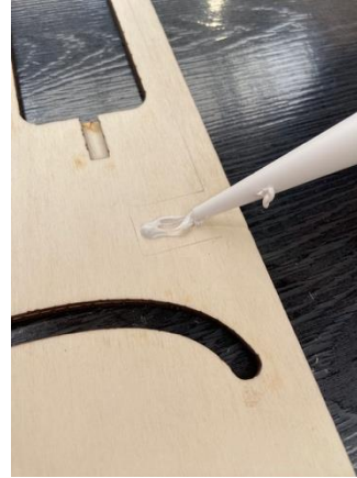
12. I couldn't use the little screws on the activity board because they would of went all the way through, so I had to use instant nails instead.
