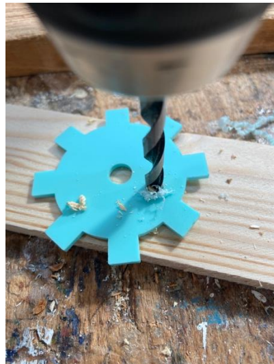
Then I proceeded to drill the hole using a 6mm drill bit.
