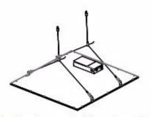
Hook mounting cables in the allocated slots Adjust cable to the desired suspension height
