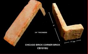
Item # CB1018U - Brickera Corner Brick. Chicago Brick Corner Veneer. The brick is used for Wall Veneer Applications, Kitchen Back Splash, Fire Places, Chimneys, BBQ's, Columns and many other applications. You will require 4 Corner Bricks per Linear Foot.
