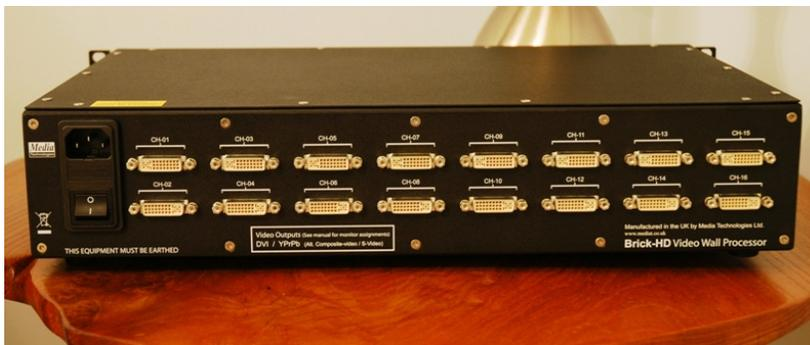
The Brick-HD is packaged in a robust welded steel 19-inch / 2U enclosure with removable feet and brackets. It can be rack mounted or free standing.
