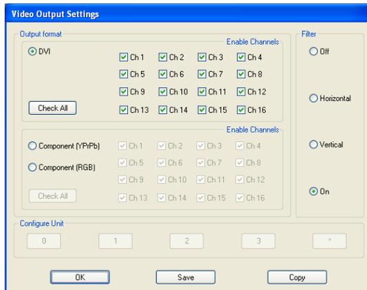
If supported by the installed firmware each output has a 2 dimensional pixel interpolation filter. This can be enabled or disabled in both directions independently. If the installed firmware version does not support the interpolation filter, these options will also be greyed out.
