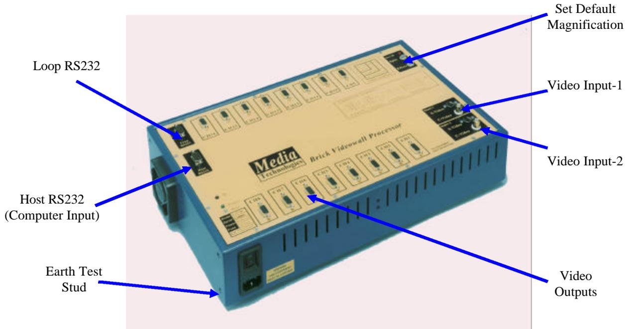
The default magnification can be changed using the 'Split' switch. Split=0 is invalid, Split=1 selects full frame video on each monitor. Split=2, selects 2x2, Split=3 selects 3x3, Etc. Connect your monitors according to the mapping shown below.
