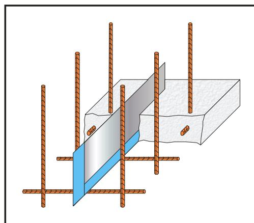
In addition to the *FERROQUELL I* standard there is a *FERROQUELL II* special version available with all-round hydrophilic rubber coating.
