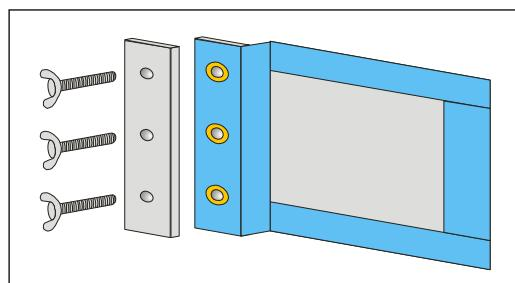
The connection of *FERRODEHN* to the *FERROQUELL*-system is achieved by using standard fixing clamps or fastening clips.
