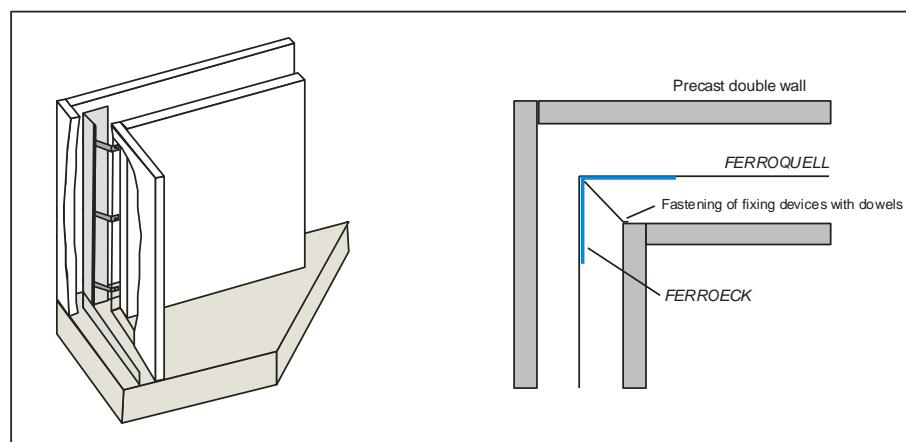
In the corner of horizontal sealing the factory-bended *FERROQUELL I* corner element (or *FERROQUELL II* corner element) should be used for an optimal connection to *FERROECK* vertical joint element.
