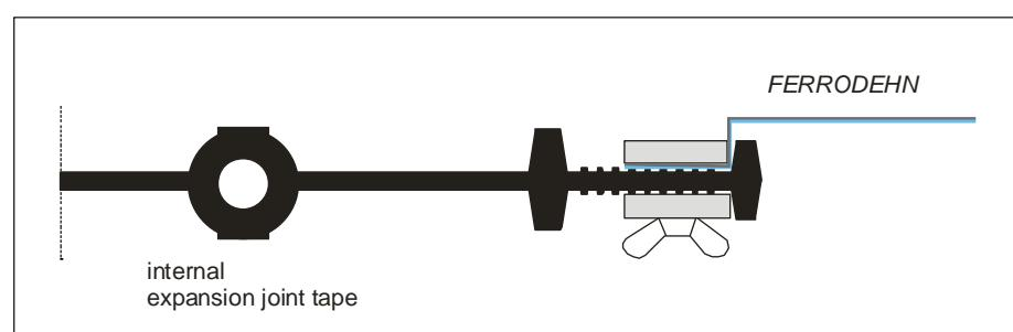
The fixation to expansion joint tapes is carried out by means of a flange connection, which can be fixed easily without any tool by using wing bolts. The flange is sealed with two stripes of hydrophilic rubber on both sides.
