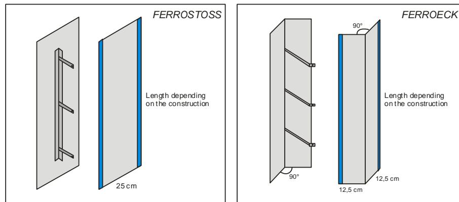
*FERROSTOSS* and *FERROECK* vertical joint elements are placed on the base plate and connected to the horizontal *FERROQUELL* joint metal waterstop each with two fixing clamps type VF. Furthermore the fixing devices of *FERROSTOSS* and *FERROECK* are fastened with dowels to the precast double wall.
