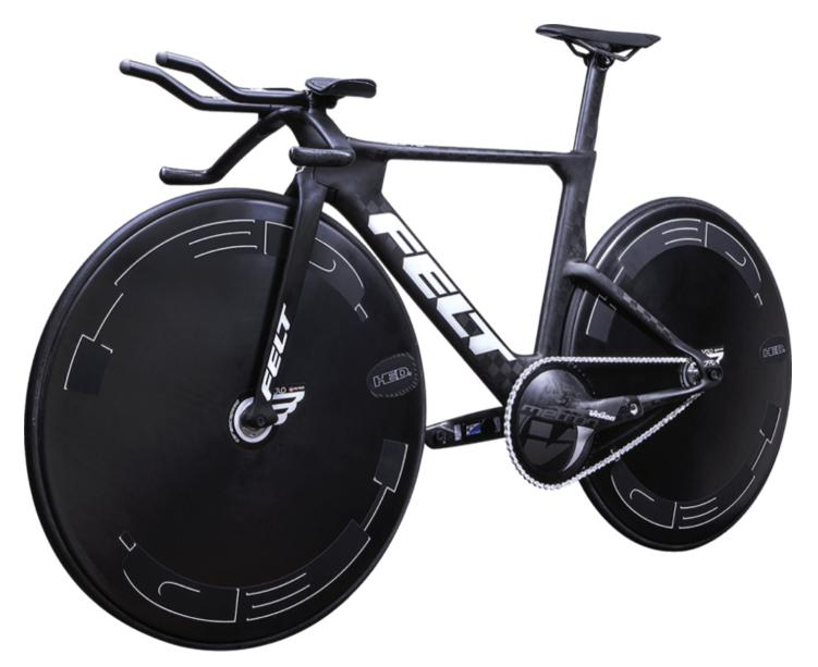
FRAME / FORK Felt TrackAero | UHC Ultimate + TeXtreme carbon fiber
