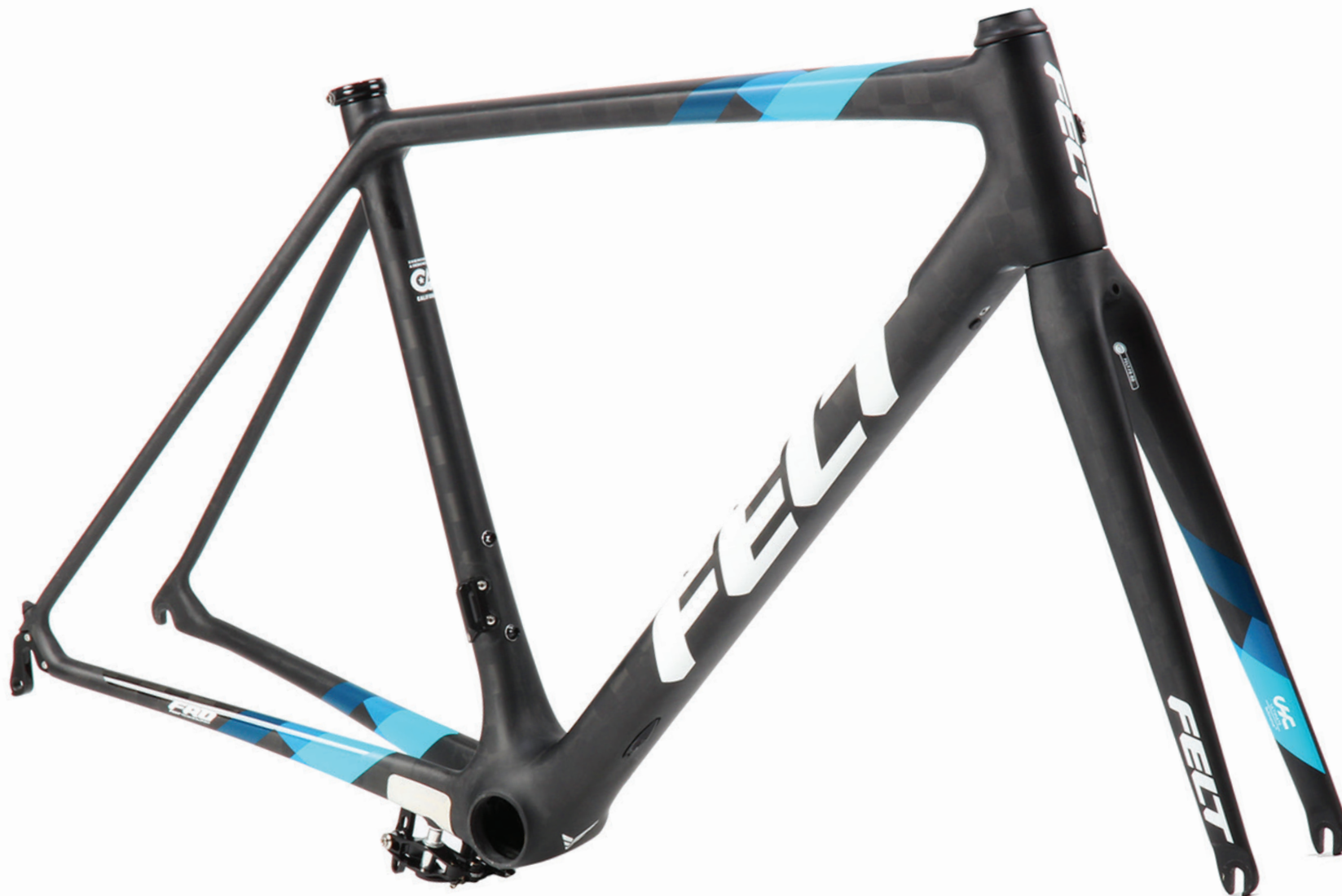
FRAME / FORK Felt Road 3.0 | UHC Ultimate + TeXtreme carbon fiber
