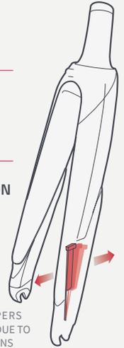
TUNED MASS DAMPERS REDUCE VIBRATIONS DUE TO ROAD IMPERFECTIONS
