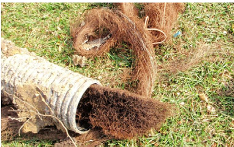
Tree roots that clog perforated pipe are a common cause of drainage failure on golf courses, especially in sites where willows, cottonwoods, and other shallow-rooted trees have been planted.
