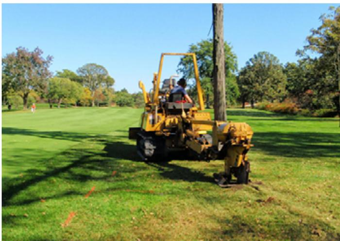
A heavy-duty vibratory plow can make quick work of severing tree roots without causing significant damage to turf. A rolling operation over the plow slit will make most surface disruption disappear. Be sure to locate and mark irrigation and underground utilities prior to root pruning operations.
