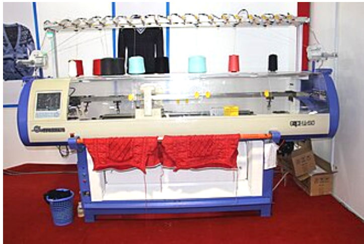
Automatic computerized flat knitting machine (Jacquard), 2017. Production machine.
